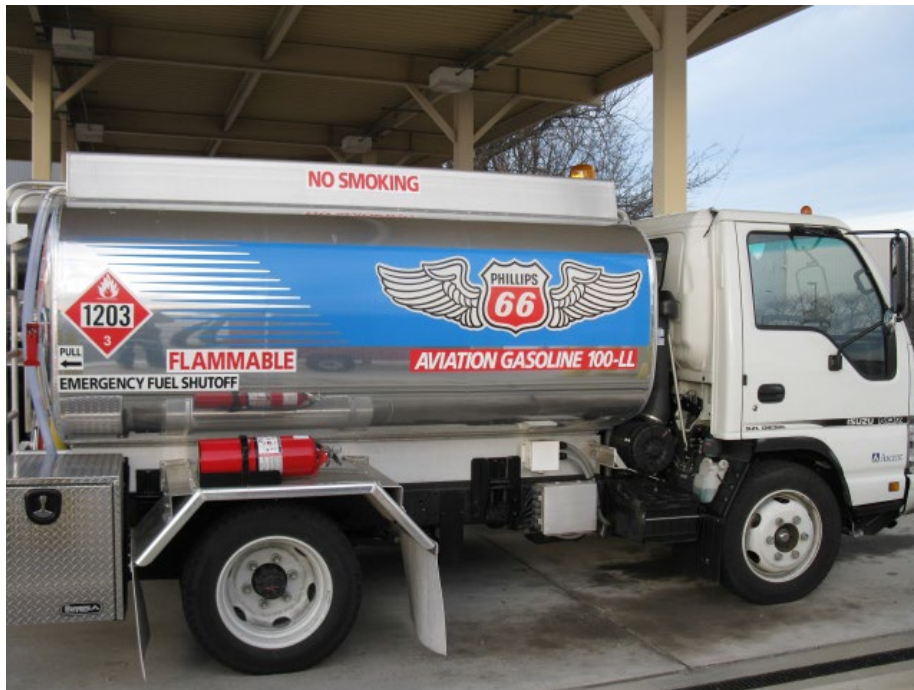
One of Two 1,500-Gallon Aviation Gasoline Tank Trucks (4407 and 4408) Parked Between Terminal and Self-Fueling Pumps
