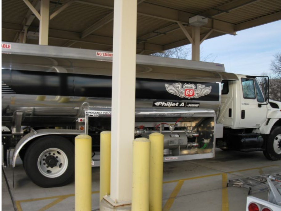
One of Two 5,000-Gallon Jet A Fuel Tank Trucks (5559 and 5560) Parked Between Terminal and Self-Fueling Pumps
